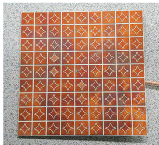
FIGURE 11. Front view of fabricated 9 \times 9 WG-CSRR array [90].
